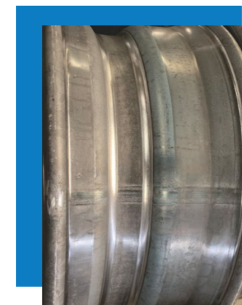
某钢企产品颜色不均 Poor quality of a product from another manufacturer
