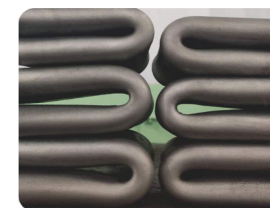
敬业440CL厚度5.95mm 纵、横向双面折叠冷弯 Longitudinal and transverse double-sided cold folding of Jingye 440CL thickness: 5.95mm
