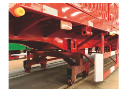
敬业700L半挂车大梁组装 Jingye 700L semi-trailer truck stringer assembly
