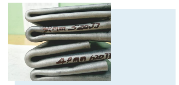
尖角折叠冷弯特性： Cold folding characteristics of sharp corners:
