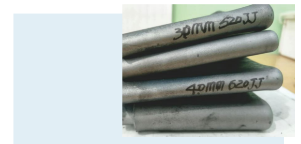
敬业520JJ、620JJ卷板纵、横向双面折叠冷弯 Longitudinal and transverse double-sided cold folding of Jingye 520JJ and 620JJ rolled plates
