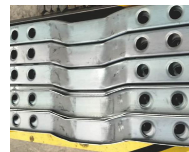
敬业700L厚度2.75mm 半挂车贯穿梁 Jingye 700L semi-trailer through-beam thickness: 2.75mm
