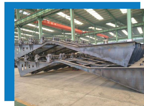
敬业620JJ水泥散装罐车体主梁(700L)结构 Bulk Cement tank body main beam (700L) structure welded with Jingye 620JJ
