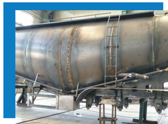
敬业620JJ水泥散装罐车体拼焊 Bulk Cement tank body welded with Jingye 620JJ
