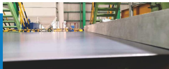
敬业600XT厚度2.5~2.75mm板面光亮平直 Bright and smooth surface of Jingye 600XT with thickness of 2.5~2.75mm
