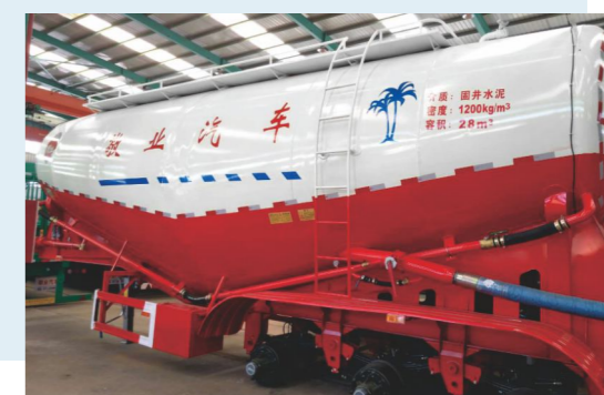
敬业620JJ水泥散装罐车体主梁(700L)结构 Bulk Cement tank body main beam (700L) structure welded with Jingye 620JJ
